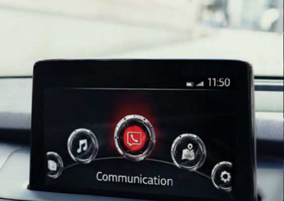
Mazda Connect 9-inch TFT LCD multi-information touchscreen display.
