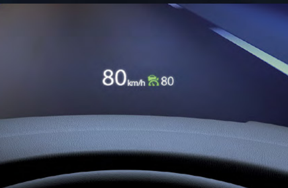
Active Driving Display is projected onto the windscreen in full colour, displaying trip information in your line of sight.
